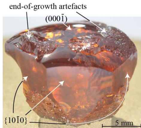
Fig. 7: AlN single crystal; homoepitaxially grown on a (000\bar{1}) -oriented wafer with 8 mm in diameter. The surface artefacts results from a touch of the growth interface with the source material at the end of the growth run.
